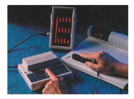
Figure 2: Optacon incorporates OCR with tactile Braile feedback
